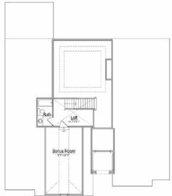
Second Floor Plan Opt. Loft: 161 SQ. FT. Bonus: 287 SQ. FT. Total: 438 SQ. FT.
